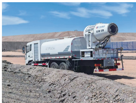
Windbreak and dust-suppression netting and Sprinkler systems
